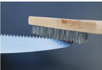
Wire brush can get in the narrow gaps between the saw teeth to remove anything stuck there.
