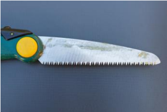
Pruning saw blade with hard-to-remove tree sap.
